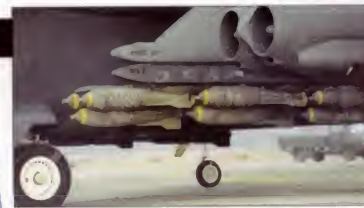
'Buffs' can mount up to 24 340-kg (750-lb) or 454-kg (1,000-lb) high-explosive or cluster bombs on external wing pylons.
